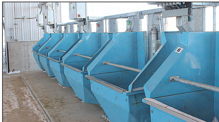
The Insentec feeding system provides amount of consumption, time of day, amount of time spent in the feeder and the number of visits to the feeders and waterers.
