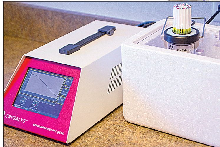
This machine can freeze up to 60 embryos by slowly cooling them to -32 °C over a period of 53 minutes.
