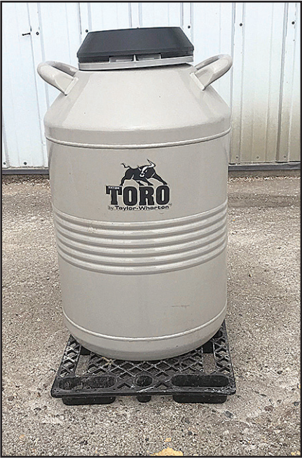
Semen Tank Storage — Cryogenic containers (Semen Tanks) should be stored in a well-ventilated room with a hard surface floor on a wood or plastic pallet. Keeping the tank off the floor will add to the tank life. There should also be adequate access for the person servicing the tank explains Gerald Feikema, Brookings, SD. (Photo from Gerald Feikema)
