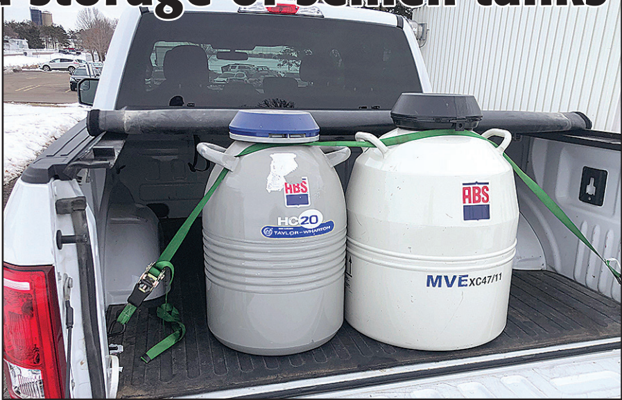
Transporting Semen Tanks - Liquid nitrogen tanks must be securely tied down in the bed of a pick-up truck when transporting. (photo from ABS Global)
